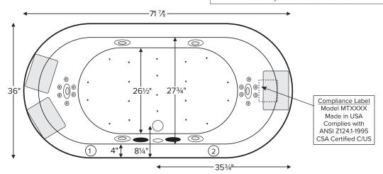
Numbered areas on tub deck represent possible locations to install cleaning systems, faucets and other fixtures. When Fill-Flush is ordered and location 2 is chosen, the detergent feeder will need to be offset to the left or the right. Shown with Air Massage and Ultra Whirlpool Package.
